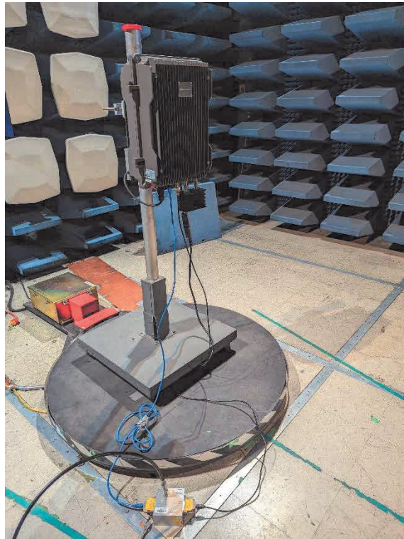
Figure 82: Conducted Emissions: Telecom Measurement Setup
