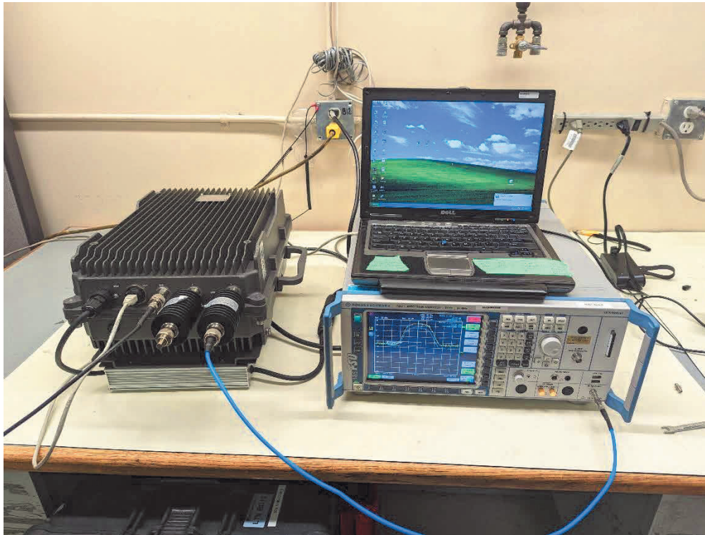
Figure 80: RF Conducted Measurement Setup
