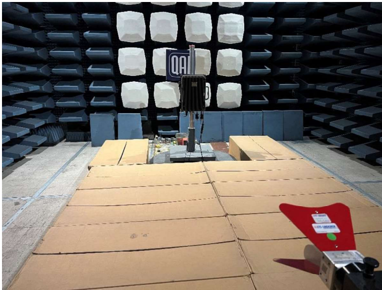
Figure 4: Radiated Emissions 1GHz to 18 GHz
