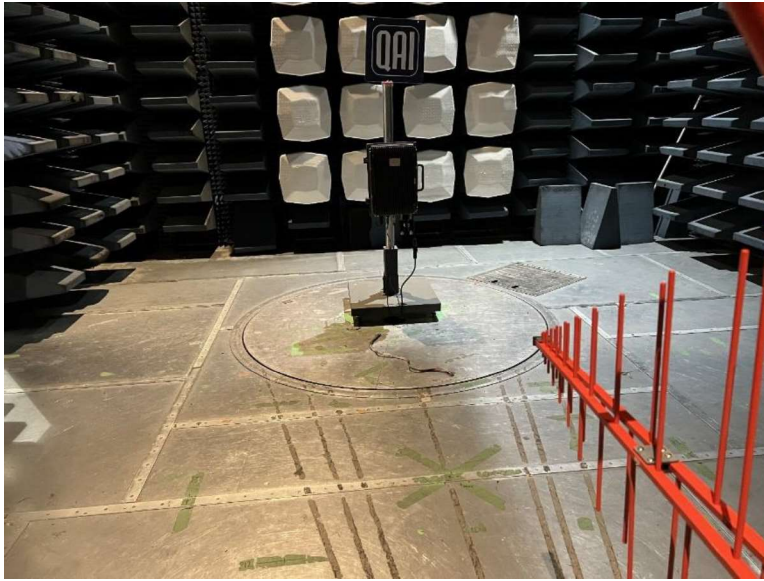
Figure 3: Radiated Emissions 30MHz - 1GHz.
