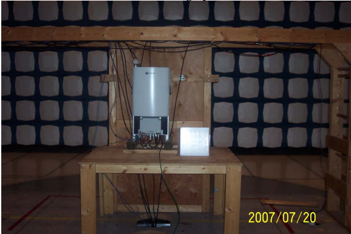
Figure 1 Radiated Emissions Test Photograph
