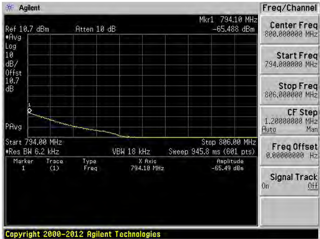
FCC Rule Part 27.53(c). Uplink. Band 13. 794 MHz to 806 MHz
