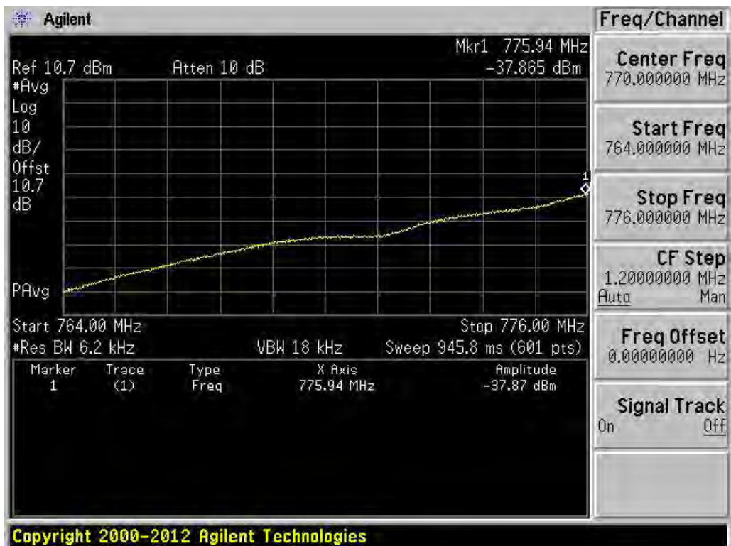
FCC Rule Part 27.53(c). Uplink. Band 13. 764 MHz to 776 MHz
