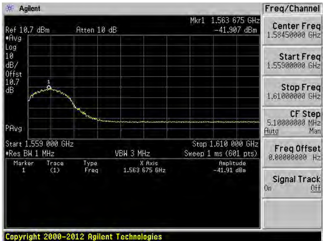
FCC Rule Part 27.53(e). Uplink. Band 13. 1559 MHz to 1610 MHz
