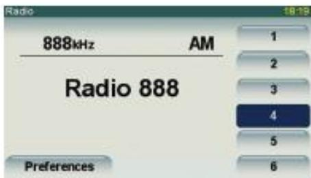
You can save a station to a preset station. There are 6 presets per radio band. To save a frequency, press and hold the number that you want to use to save the frequency. When the color of the button changes, the frequency is saved.
