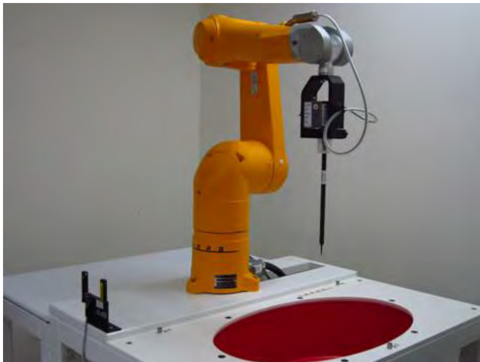
Fig.1 Photograph of the SAR measurement system
