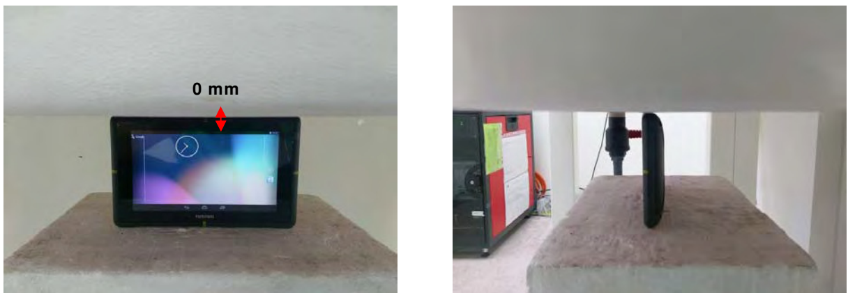
Fig.4 EUT Top side to flat phantom
