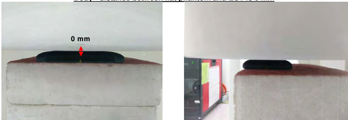
Fig.3 EUT Back side to flat phantom
