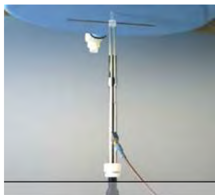
Photograph of the dipole Antenna
