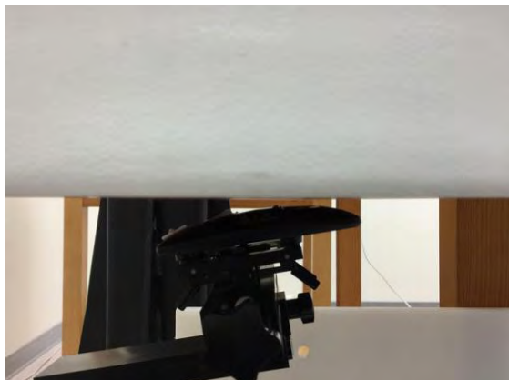
Fig.6 EUT Curve side to flat phantom
