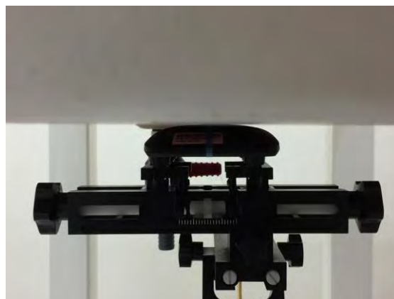
Fig.3 EUT Back side to flat phantom
