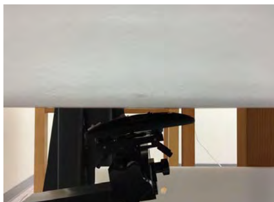
Fig.6 EUT Curve side to flat phantom
