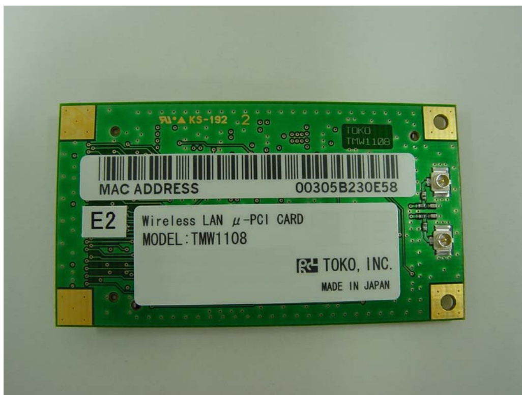
Front of WLAN Module
