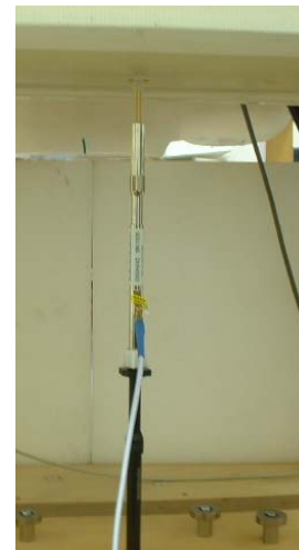
5100-5800MHz Systemperformance check setup
