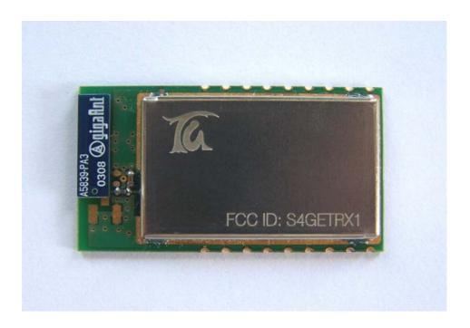
Also a label will be placed on the top surface of the ETRX1 Module RF shielding can showing our batch coding identification, as shown in **Figure 2**.
