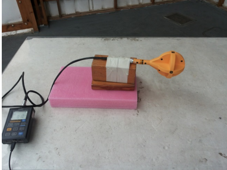
Photograph 7.1.1 Setup for RF exposure measurements, noise measurements
