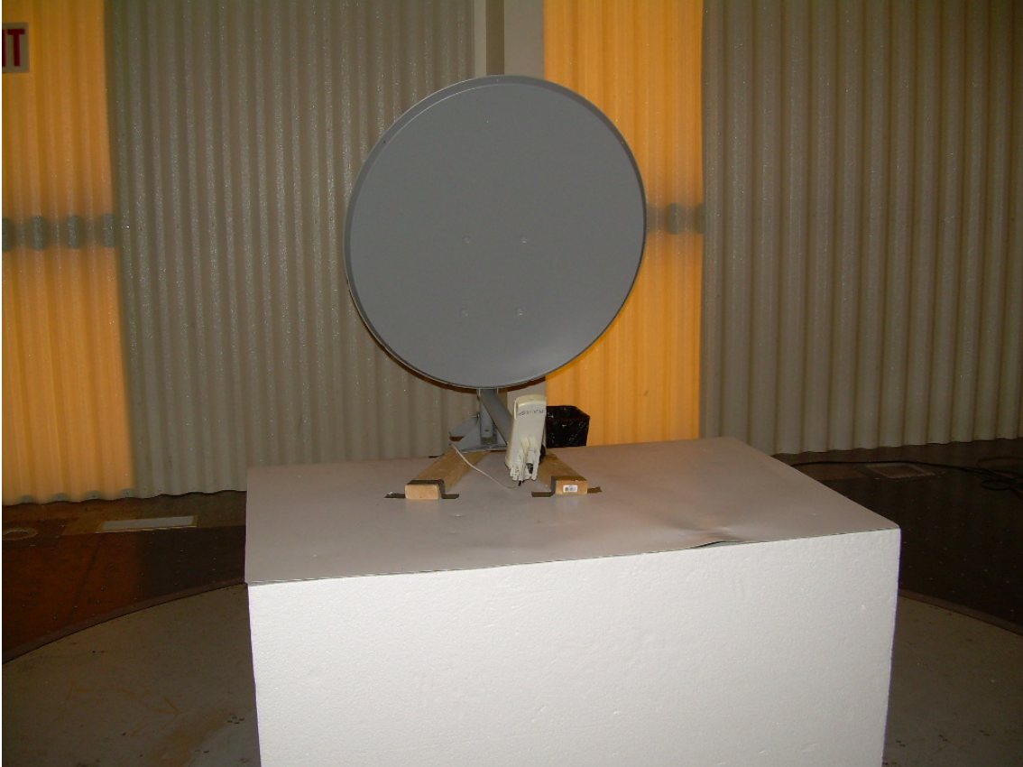
Photograph 5 – Front View Radiated Disturbance – RCL-3 Antenna
