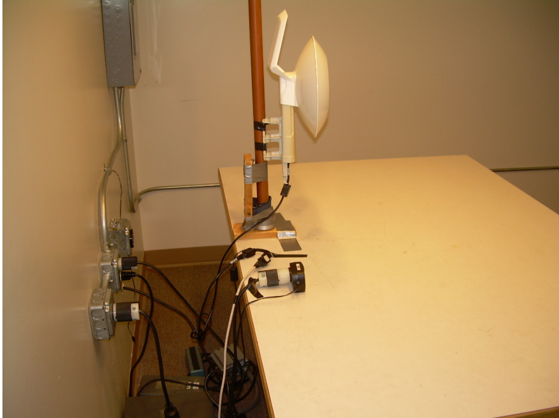
Photograph 8 – Back View Conducted Disturbance Test Setup
