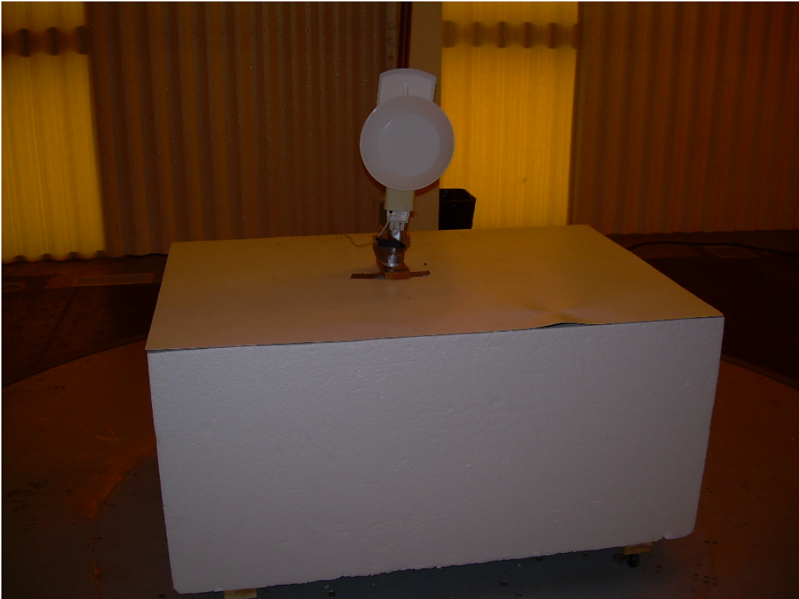
Photograph 1 – Front View Radiated Disturbance – Classic Stinger Antenna
