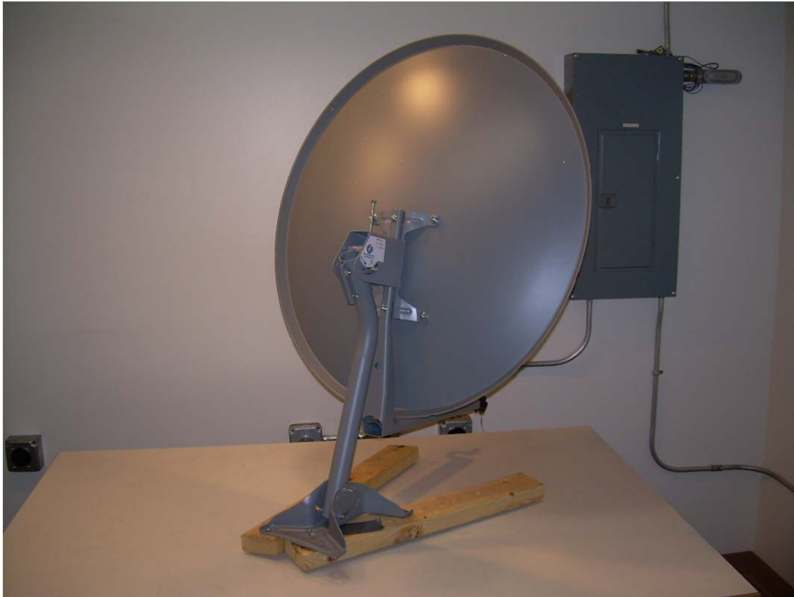
Back View of the RCL-3 Antenna
