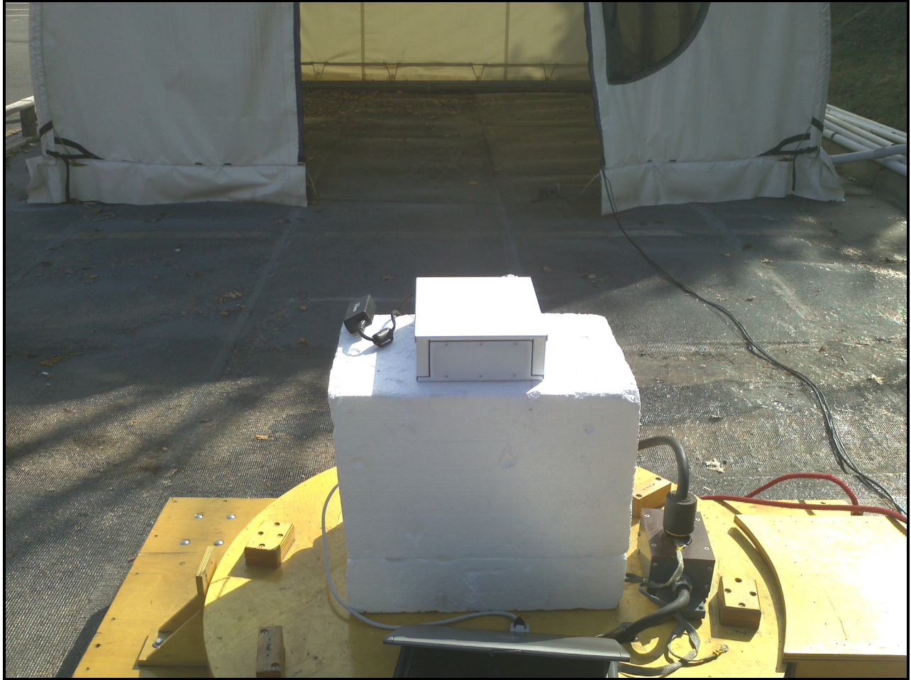
Photograph 18: Radiated Emissions - Front View
