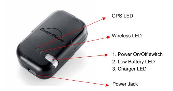
How to turn on the BT-R900: Continued press power button 3 seconds. How to turn off the BT-R900: Continued press power button 3 seconds or automatic turn off.
