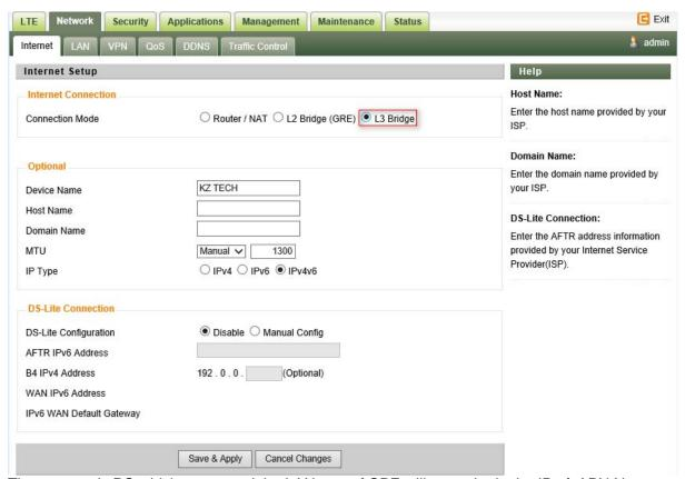
The operator's PC which connected the LAN port of CPE will auto obtain the IP of APN Net when the CPE attached to the APN network, then you can connected to the APN network for data services. And the PC should configure a static IP address as 10.1.1.x manual in order to visit the CPE managing page <a href="http://10.1.1.1">http://10.1.1.1</a>.
