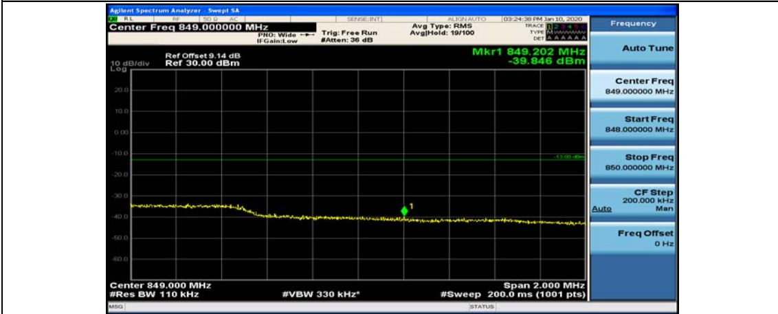
Channel Bandwidth: 10 MHz_HCH_QPSK_25RB#12
