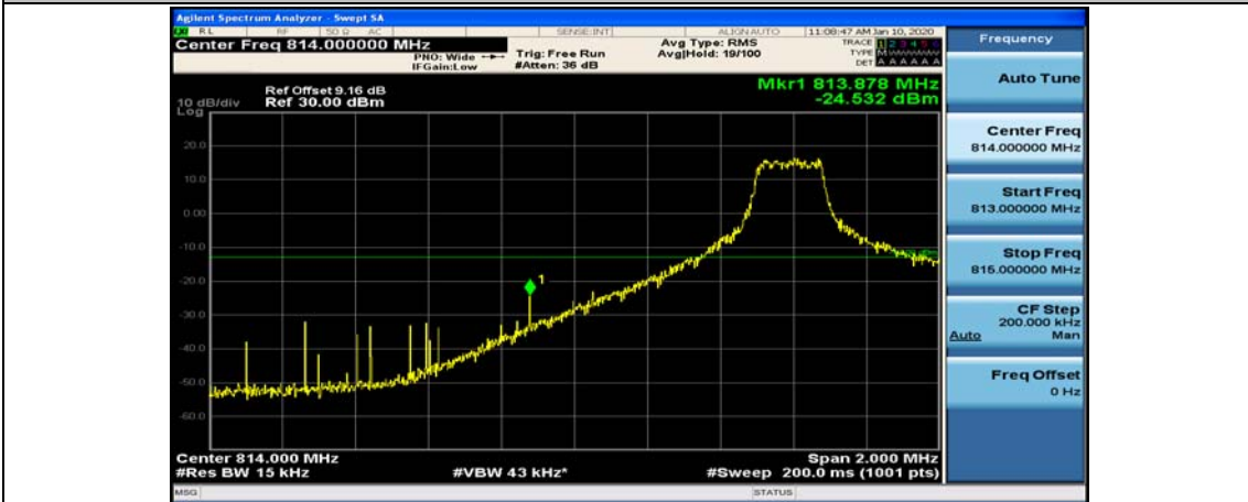
Channel Bandwidth: 10 MHz_MCH_16QAM_1RB#24
