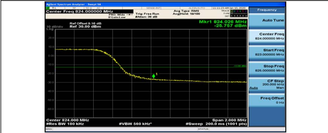
Channel Bandwidth: 10 MHz_MCH_QPSK_50RB#0
