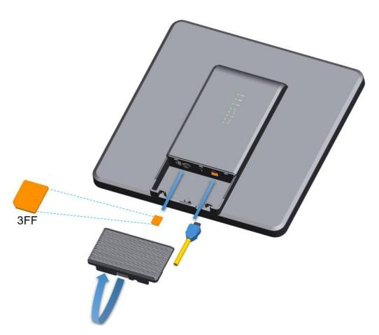
Open the cover, insert the SIM card and connected the ETH cable.
