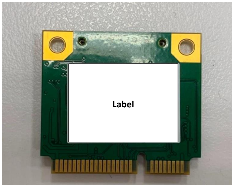
Rear side of the RF module
