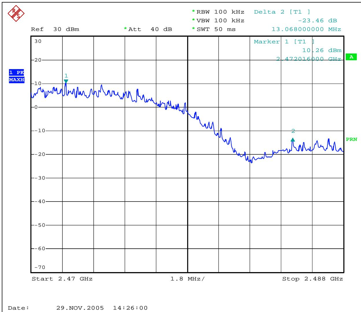
**3.4 Spurious RF Antenna Conducted Emissions, FCC 15.247(d)**
