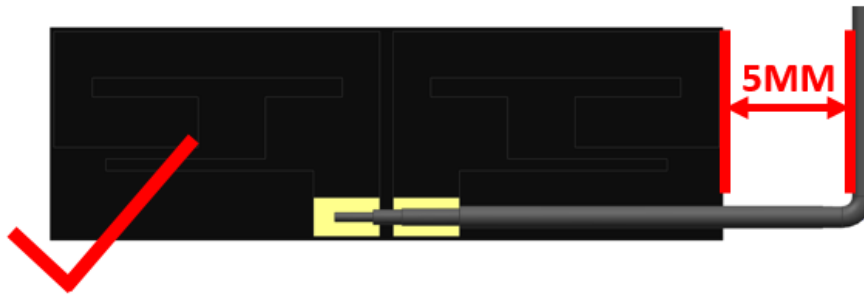
FIGURE 5.2.1 RECOMMENDED CABLE BENDING RANGE
