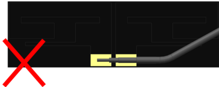
FIGURE 5.2.2 UNRECOMMENDED CABLE BENDING
