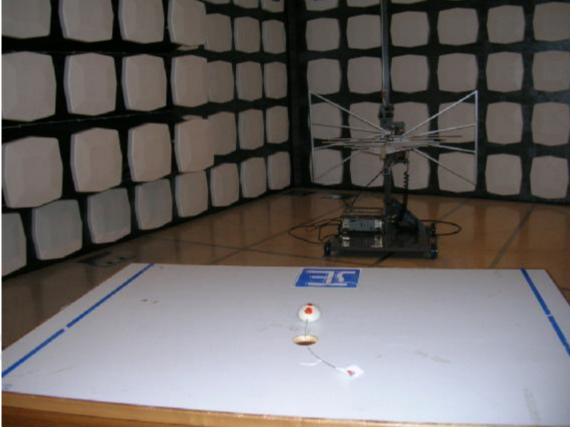
Measurement of Radiated Emission Test Set Up
