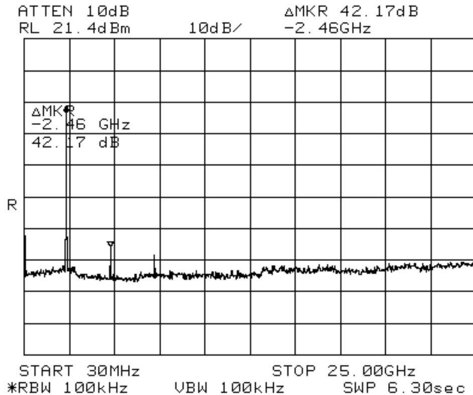
**Test Data – Spurious Emissions at Antenna Terminals**
