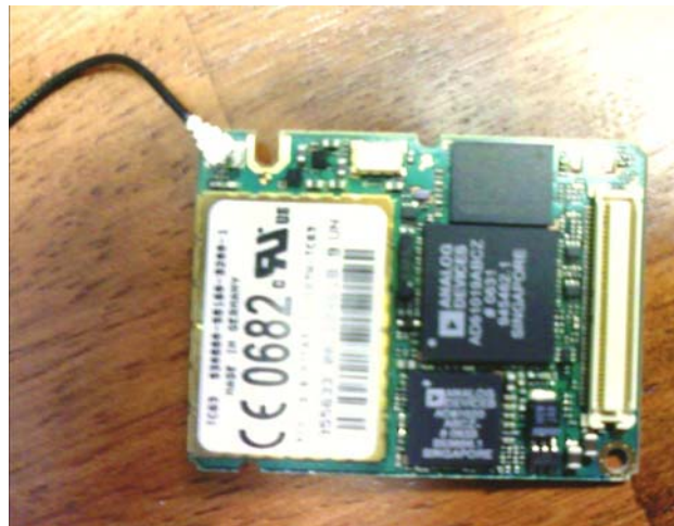
TC63 cellular radio module
