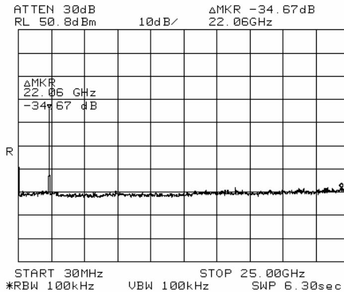
**Test Data – Spurious Emissions at Antenna Terminals****Mid Channel**
