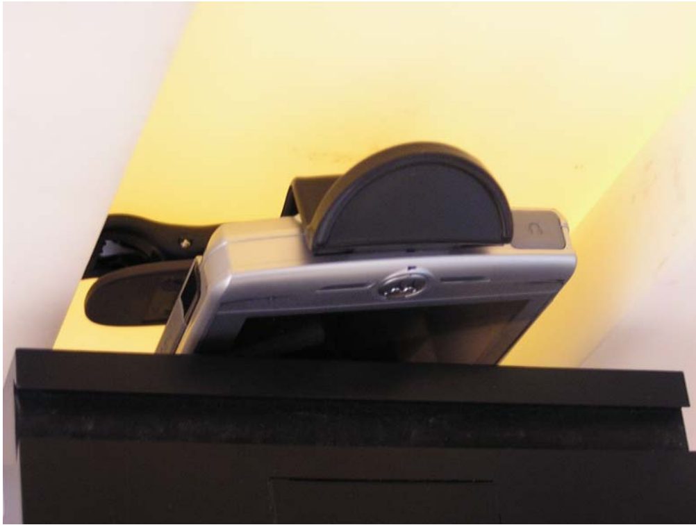
Figure 5: Phone Against the Flat Phantom with Holster
