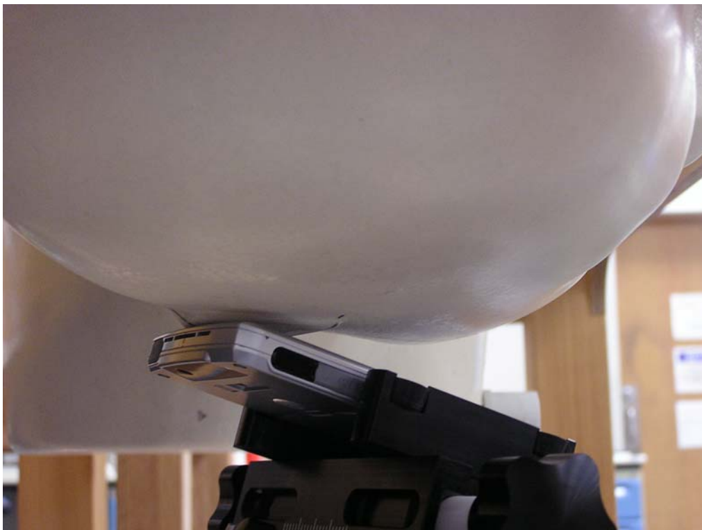
Figure 4. Phone Against the Head Phantom (15°Tilt)
