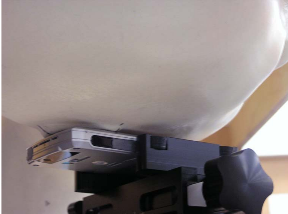
Figure 3. Phone Against the Head Phantom (Cheek Touch)
