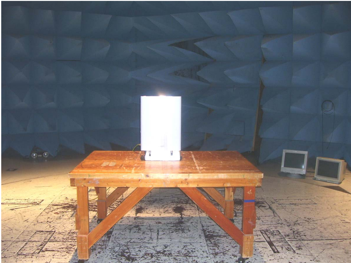
Photograph 4. Radiated Emission Limits Test Setup – Front View
