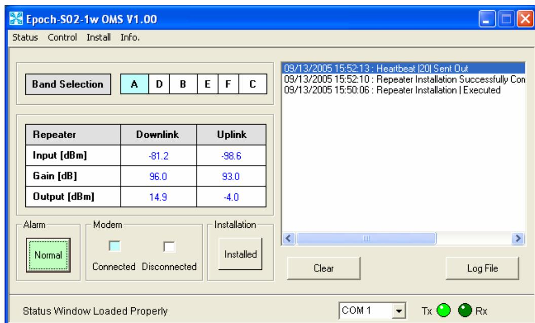
3. Check the communication port on the bottom of the GUI (Graphical User Interface) window. If you see the following prompt “COM Port 1 Successfully Opened” on the lower left portion of the window, the OMS software and the laptop can communicate with each other properly. For example, if “COM Port 1 Failed To Open” appears, choose a different Com Port as shown below until proper communication is established.
