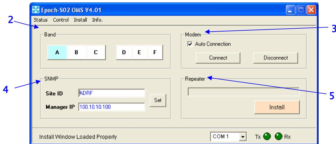
2. On the Installation screen, select the desired operating “Band.” The default is “A” Band.
