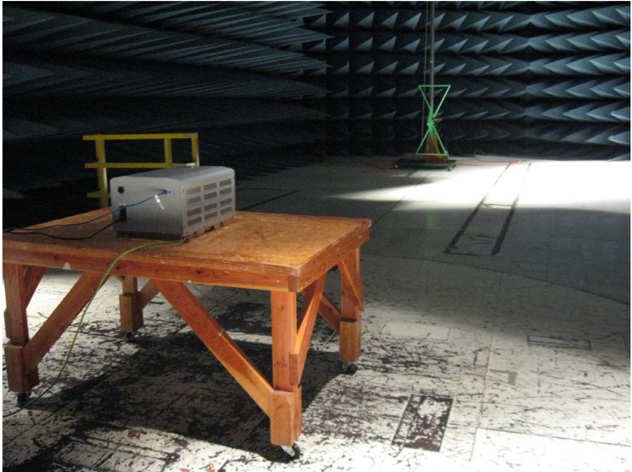
Photograph 3. Radiated Emission Limits Test Setup
