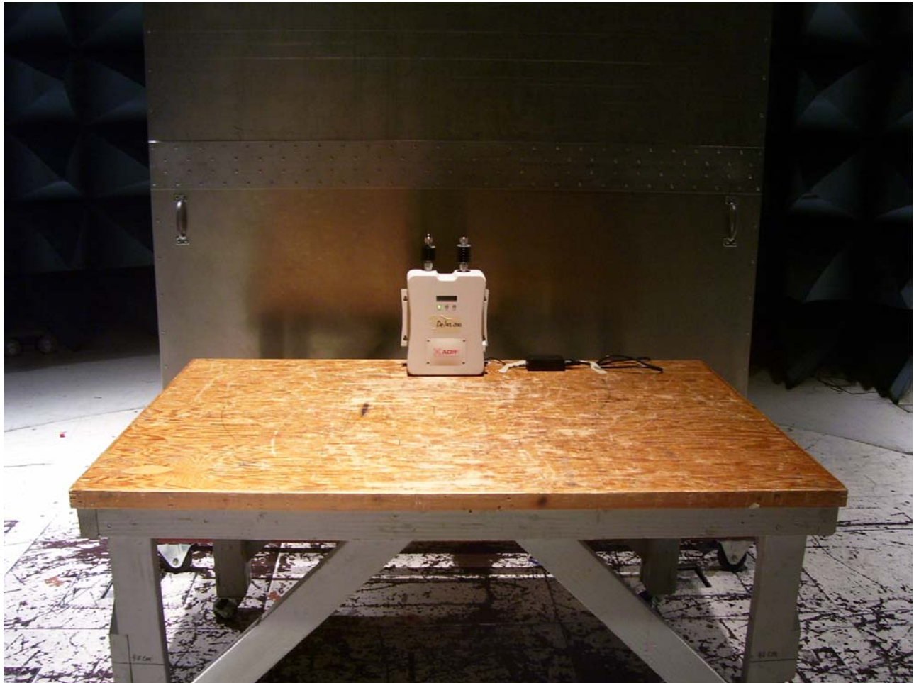
Photograph 2. Conducted Emissions Test Setup
