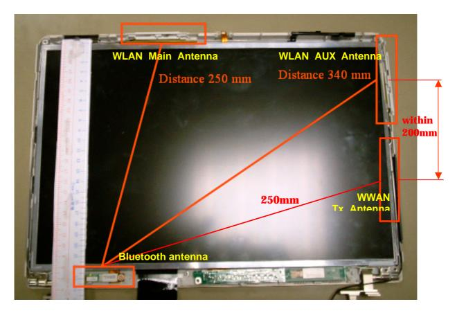
Since the Bluetooth antenna is assembled apart from the other WWAN and WLAN antennas with 25 cm or more, the co-located Bluetooth transmitter is allowed to evaluate the RF exposure compliance independently of other transmitter devices.
