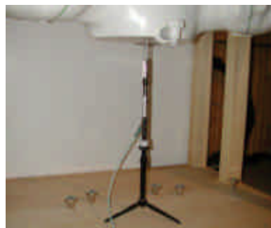
Figure A.0 Dipole Validation Test Setup
