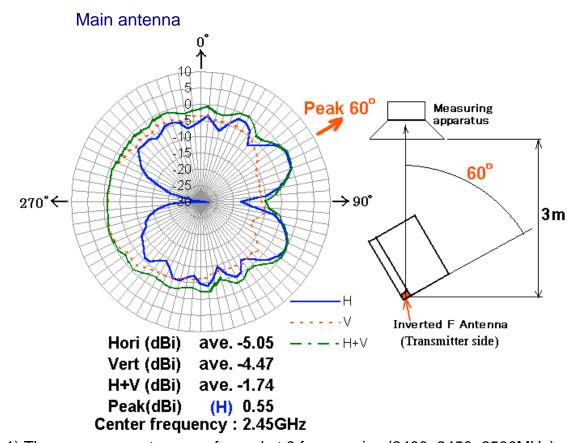
Note1) The measurement was performed at 3 frequencies (2400, 2450, 2500MHz).
