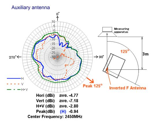
Note1) The measurement was performed at 3 frequencies (2400, 2450, 2500MHz).
