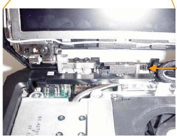
Auxiliary antenna Inverted-F type P/N: 46L6324
