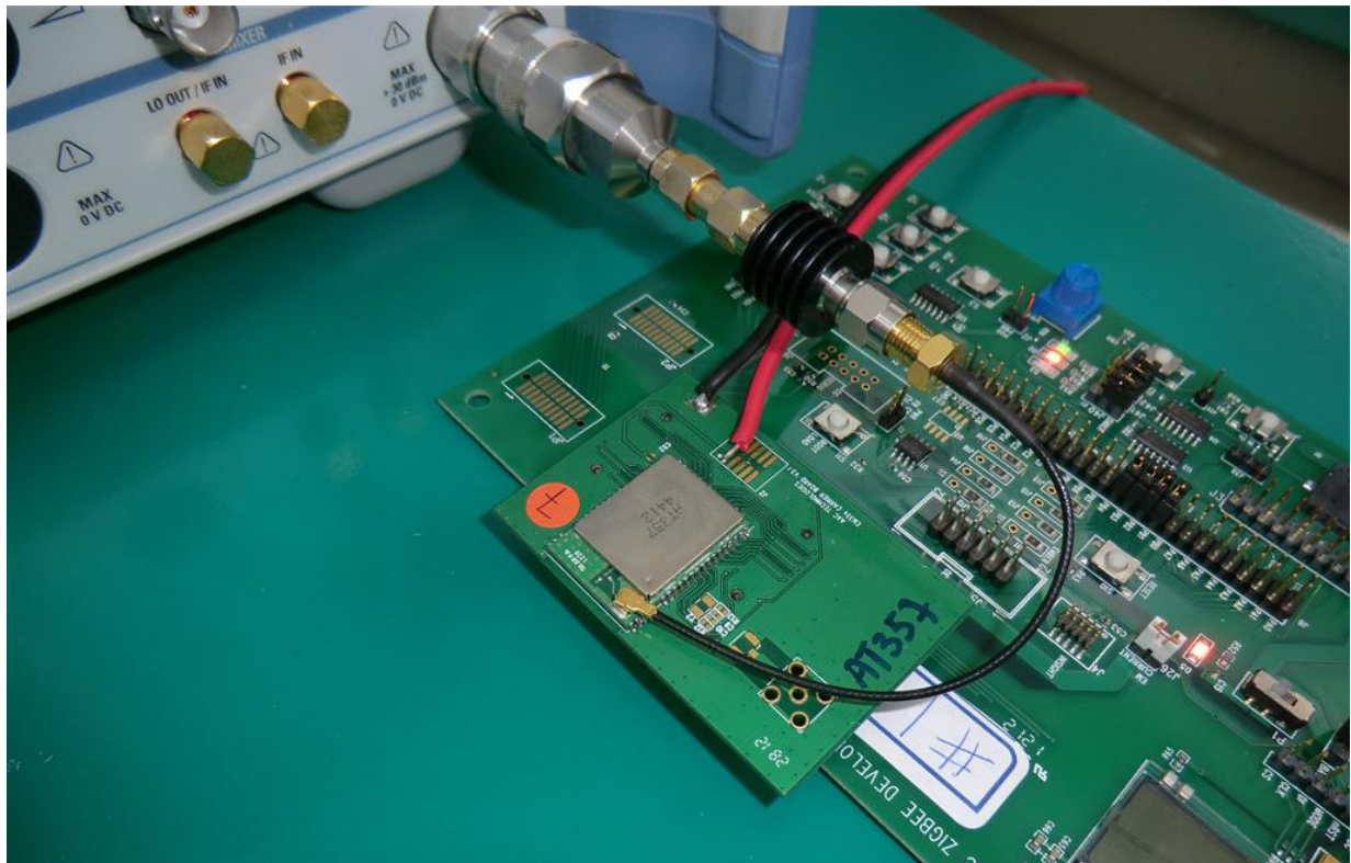
Photograph 4: Set-up for Conducted testing
