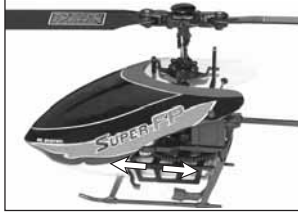
Step 1: disconnect the power cable of the helicopter.
