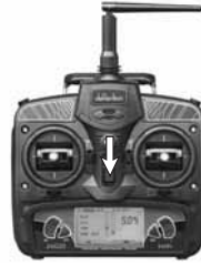
Step 2: turn off the transmitter.
