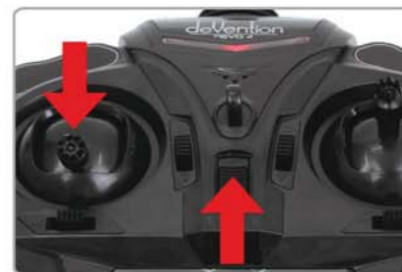
Chart 2: Pull down throttle control sticker to the lowest position and then turn on the radio.
