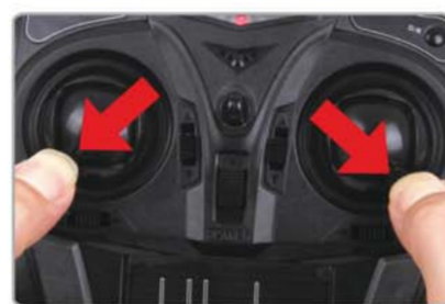
Chart 1: Enter into compass calibration, aircraft indicator will blink red and blue alternately
