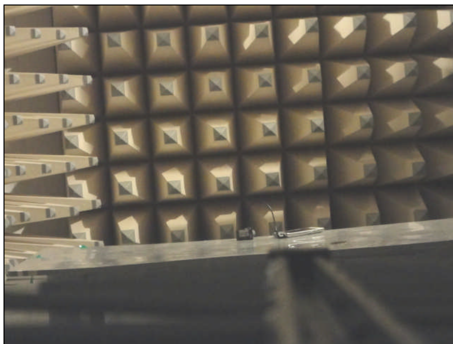
EUT on the turn table which rotate 360° during the testing to find the maximum field-strength readings
