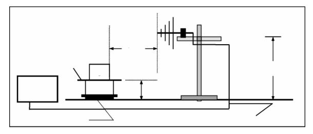
The equipment under test is placed on a non metallic table with 0.8 m height.
