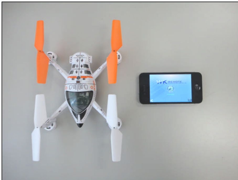
Test configuration: 1. R/C Helicopter QR W100S (with RX2646H-D module) 2. Iphone 4S with WK-REMOTE APP version 1.1
