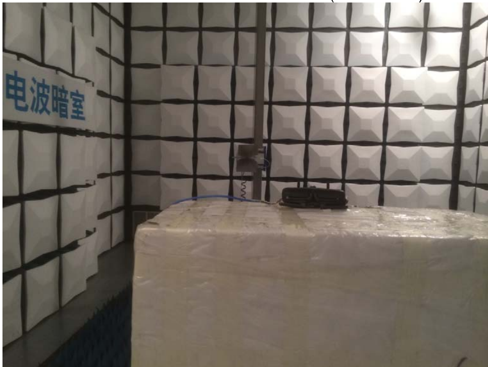
RADIATED RF MEASUREMENT SETUP (Above 1 GHz)
