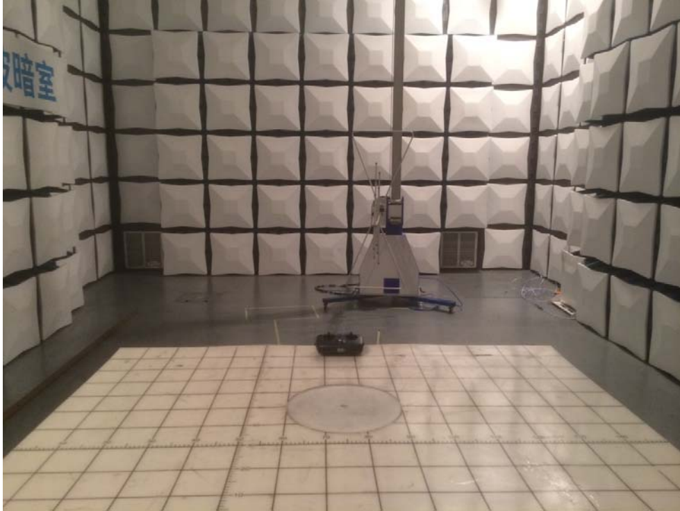
RADIATED RF MEASUREMENT SETUP (Above 1 GHz)
