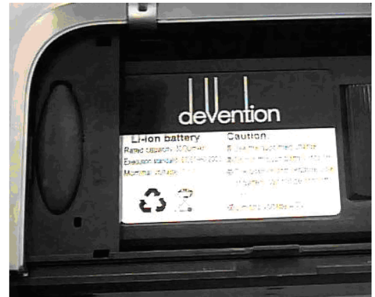
put the battery pack into the battery compartment and push it leftwards
