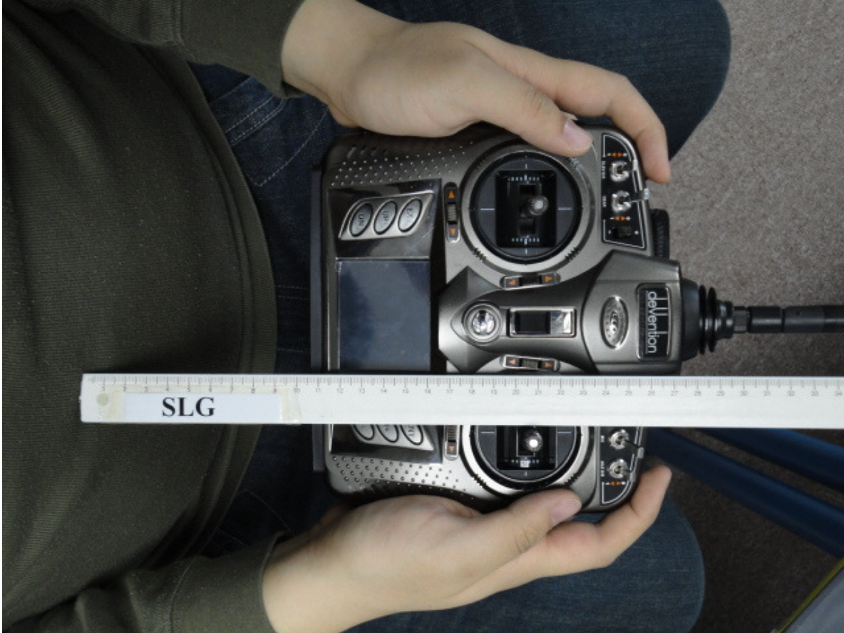
Picture1: Close to chest (29.5cm from antenna to torso) normal operation
