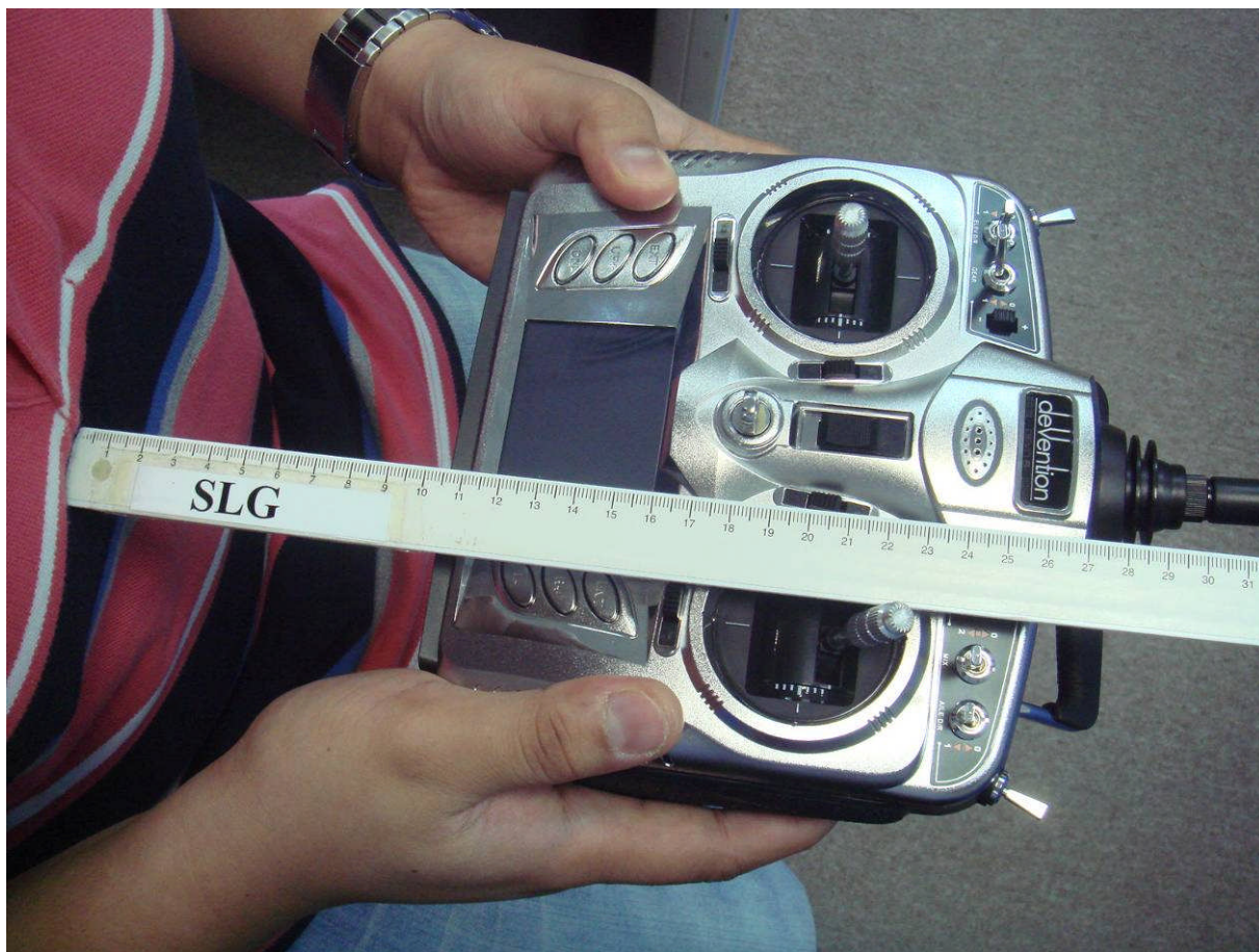
Picture1: Close to chest (29cm from antenna to torso) normal operation
