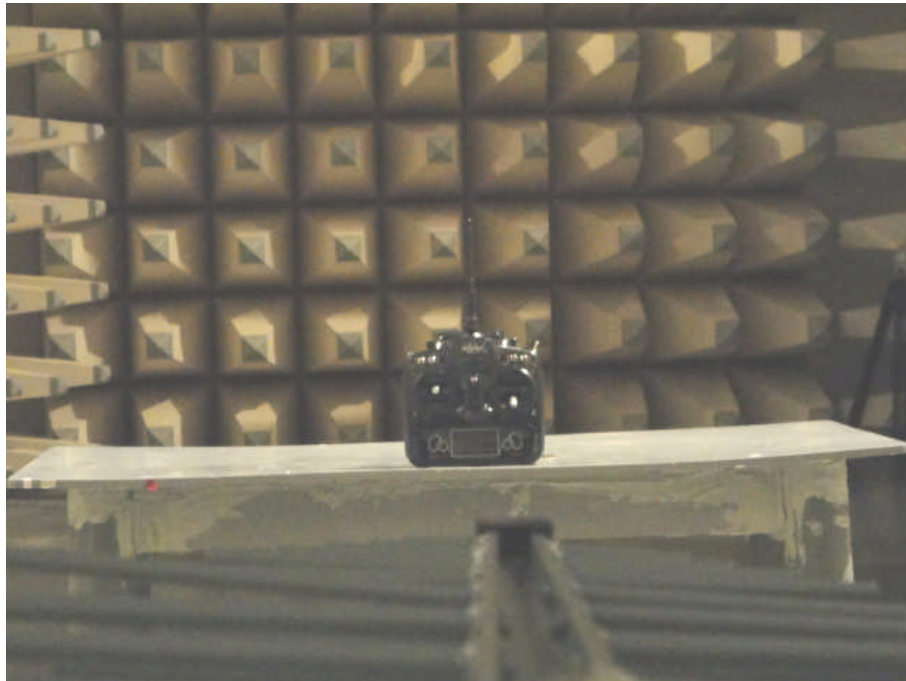
EUT on the turn table which rotate 360° during the testing to find the maximum field-strength readings
