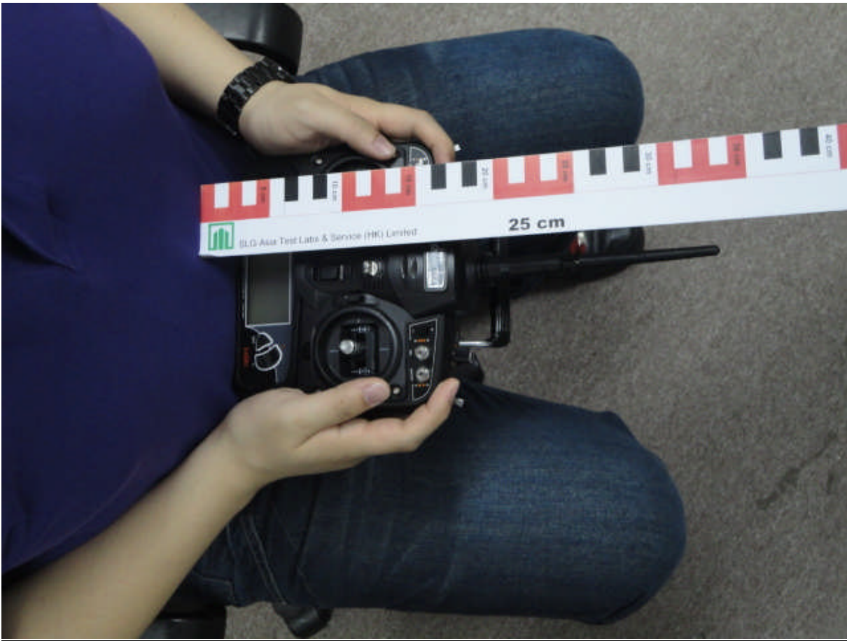
Picture2: Close to chest (20.5cm from antenna to torso) worst case operation
