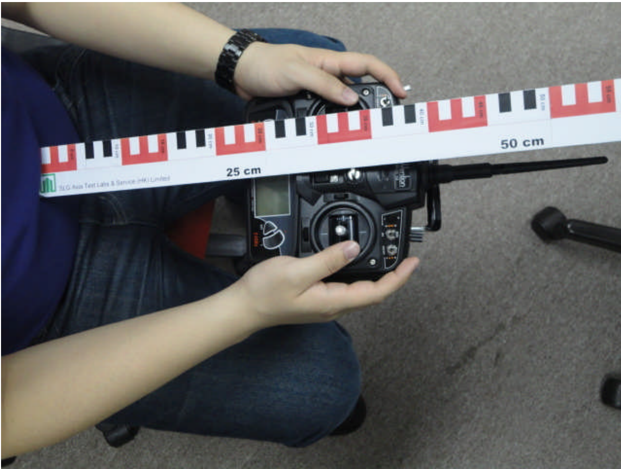
Picture1: Close to chest (40cm from antenna to torso) normal operation
